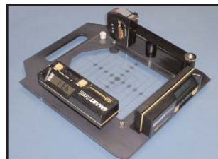
Digital tape measure locked outside the aperture when not in use.
