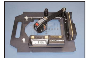
Digital tape measure swings into central axis of the beam for SSD / ODI measurements.
