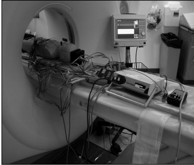
Fig. 2 —Anthropomorphic phantom of 5-year-old child positioned supine in CT gantry with metal oxide semiconductor field effect transistor (MOSFET) system and heart rate simulator.
