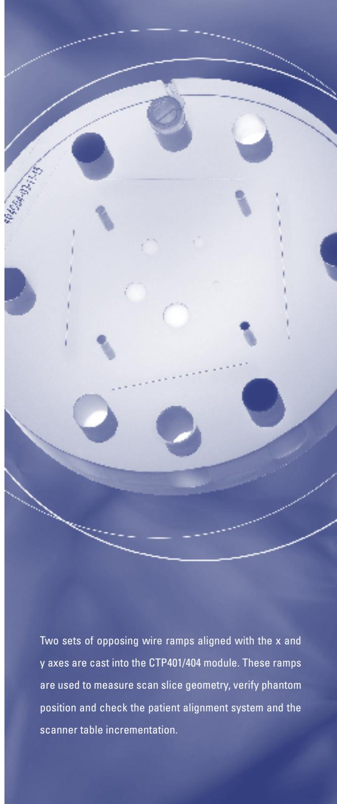
Two sets of opposing wire ramps aligned with the x and y axes are cast into the CTP401/404 module. These ramps are used to measure scan slice geometry, verify phantom position and check the patient alignment system and the scanner table incrementation.
