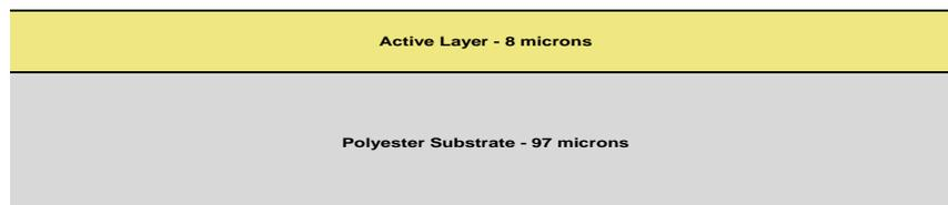
Figure 1: Configuration of GAFCHROMIC<sup>®</sup> HD-V2 Dosimetry Film
