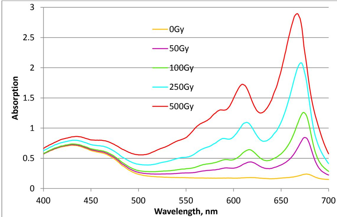
Figure 3 Spectra of GAFCHROMIC<sup>®</sup> HD-V2 as a function of adsorbed doses
